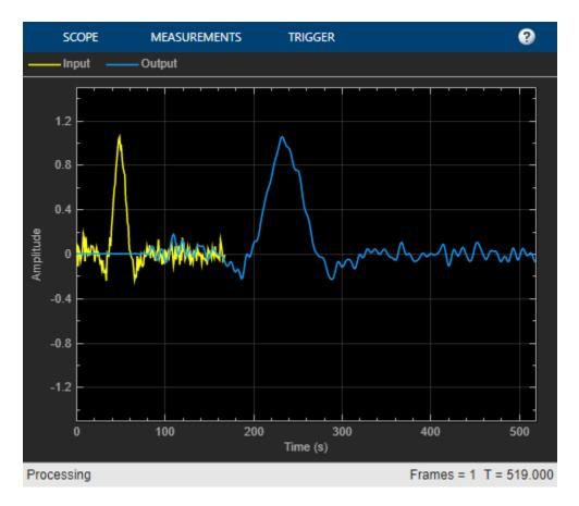
To plot the input and output signals on the same plot, you must account for the delay and the time scaling.
