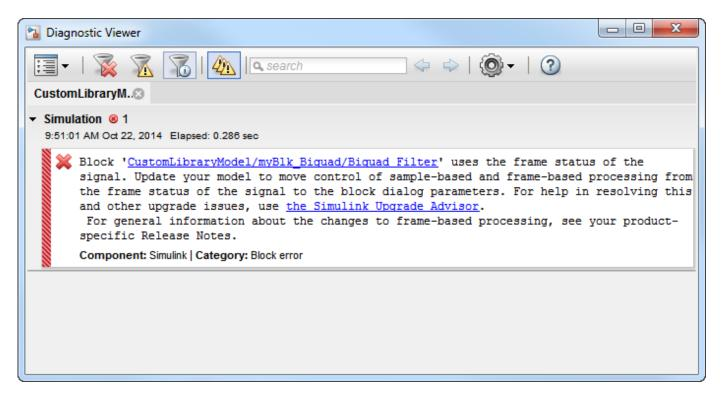
To resolve this error message, reopen Simulink Upgrade Advisor, select the Check model for custom library blocks that rely on frame status of the signal check and click **Run This Check**.
