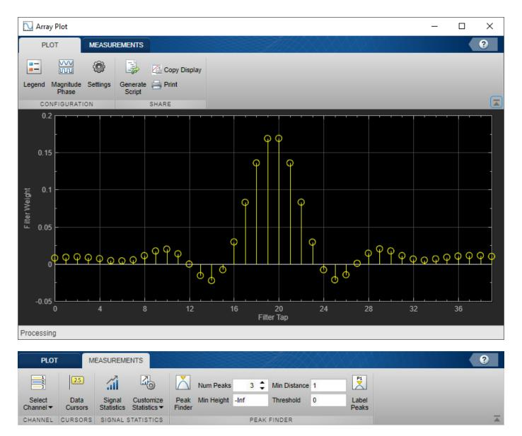
By clicking different buttons in the toolstrip, you can configure settings, turn on measurements, and share an image of the plot.
